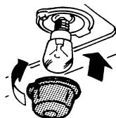
Reassemble the glass cup and reconnect the appliance.
