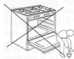
**Warning: For models with warming drawer. Never use the warming drawer to store inflammable substances that cannot withstand heat such as: wood, paper, spray cans, rags, etc...**
