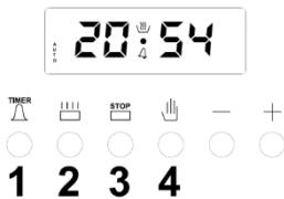
The electronic timer, which enables your oven to get the food ready to serve at the desired time. The only thing to be done is to program the cooking time and ready time. It can also be used as an alarm clock, where you just give in the amount of time after which it should remind you by a buzzer tone.
